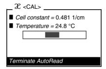
Wait for the end of the AutoRead measurement or accept the calibration value with <**MENU/ENTER**>.
