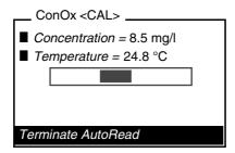
Wait for the end of the AutoRead measurement or accept the measured value with <**MENU/ENTER**>.
