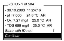
If necessary, change and confirm the ID number (1 ... 999) with  $\langle A \rangle \langle \nabla \rangle$  and  $\langle MENU/ENTER \rangle$ .
