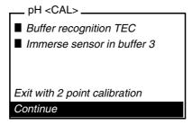
For two-point calibration, select *Exit with 2 point calibration* with <**△**> <**▼**> and confirm with <**MENU/ENTER**>.
