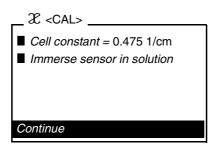
4 Immerse the conductivity measuring cell in the control standard solution, 0.01 mol/l KCI.
