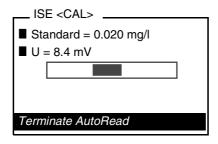
Wait for the end of the AutoRead measurement or accept the calibration value with **<MENU/ENTER>**.
