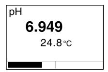
The active automatic data storage function can be recognized from the progress bar in the status line. The progress bar indicates how much of the adjusted storage duration has already expired.
