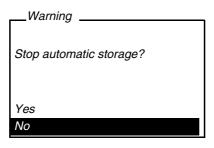
Select and confirm Yes with <**△>** <**▼>** and <**MENU/ENTER>**. The measuring instrument switches to the measured value display.
