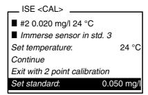
For two-point calibration, select *Exit with 2 point calibration* with <**A>** <**V>** and confirm with **<MENU/ENTER>** .
