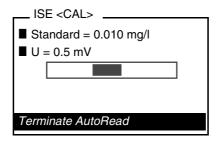
11 Wait for the end of the AutoRead measurement or accept the calibration value with **<MENU/ENTER>**.
