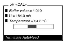
Wait for the end of the AutoRead measurement or *Terminate AutoRead* and accept the calibration value with <meNU/ENTER>.
