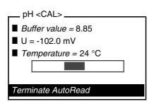
Wait for the end of the AutoRead measurement or *Terminate AutoRead* and accept the calibration value with <**MENU/ENTER>**.
