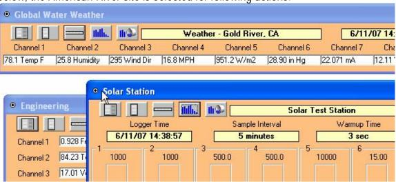
To select a data window to be active you can: Click the blue bar at the top of the desired data window, click on the radio name from the list of client radios in the address book window, select the station from the Window menu in the toolbar, or select it from the View Client Logger From List function from Client on the toolbar.
