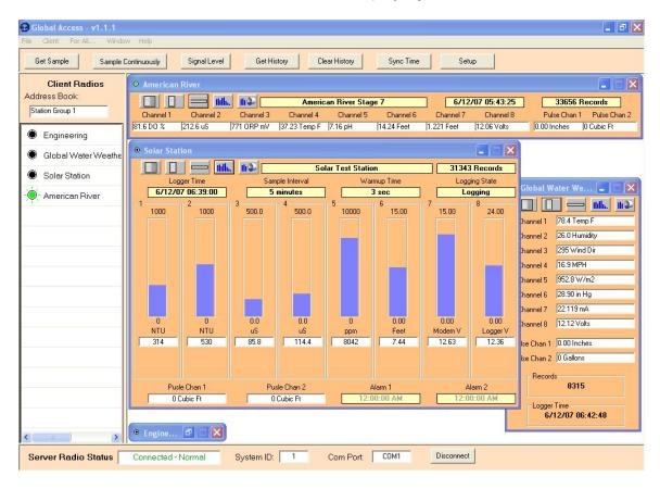
Five display modes are available, which are selected by clicking the corresponding display button in the top left of each display window.
