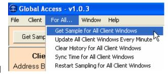
to the bottom of the screen. These operations will not be performed on loggers which are in the client list but which have not been opened at the time the operation is performed. A warning message will appear before making any critical changes and a dialog box will appear for all functions (except Update Every Minute) showing the pass/fail status of the operation on each logger .
