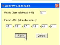
Edit Client Radio From List: Use this function to edit an exiting radio's name, channel and MAC address. Click on the client to be edited then make any necessary changes. Click Finish.
