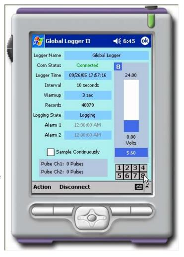
The bar graph to the right displays the status of a single analog channel. Due to the small screen size, only one channel is shown at a time. Changing the displayed channel is done by touching the channel number just below the bar graph. The channel number of the bar graph currently in the display is shown just above the top of the bar, in this case, channel 8. At the bottom of the screen are two commands, "Disconnect" will disconnect from the logger, while "Action" access other functions.
