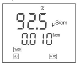
4 Confirm the selection with **<OK>**. The meter switches to the measured value display.
