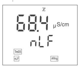
4 Confirm the selection with **<OK>**. The nonlinear temperature compensation is switched on. The meter switches to the measured value display. The selected temperature compensation appears as the status display.
