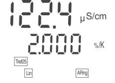
4 Set the temperature coefficient with  $< \Delta > < \nabla >$ , e. g. 1.880 %/K.
