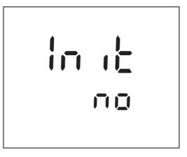
3 Press <▲><▼> to display *no* or *YES*. *YES*: Reset the meter settings. *no*: Retain the meter settings. Confirm with <**OK**>.
