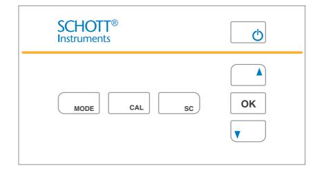
In this operating manual, keys are indicated by brackets <..> . The key symbol (e.g. **<OK>**) generally indicates a short keystroke (under 2 sec) in this operating manual. A long keystroke (approx. 2 sec) is indicated by the underscore behind the key symbol (e.g. **<OK\_\_>**).
