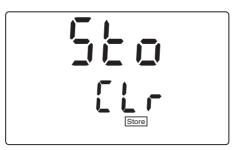
4 Confirm the clearing process with **<RUN/ENTER>**. Pressing any other key prevents the clearing, the data records will remain stored.
