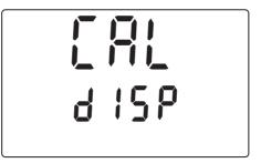
2 Press the <RUN/ENTER> key.The relative slope appears on the display:
