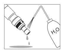
Rinse the sensor head with deionized water.
