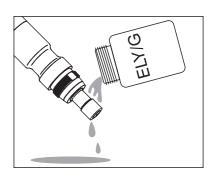
Rinse the sensor head with electrolyte solution.
